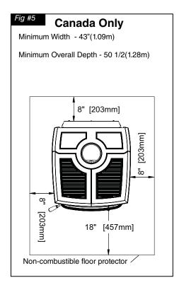
The stove may be installed on a combustible floor provided noncombustible ember protection is used.
