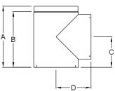
Combines a  $90^\circ$  transition with a clean out. Includes a tee cap.
