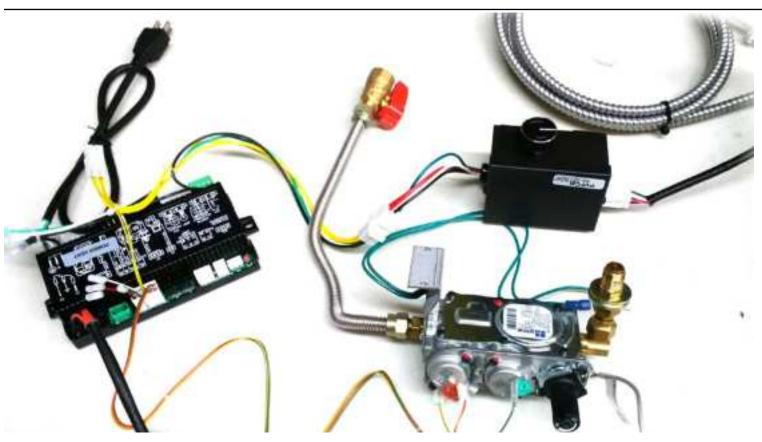
Install the PVFCB between the 6-pin Molex connector of the fireplace harness and the plug the EPVH-\*\* power cord into the mating 6-pin Molex connector in the box, as in the photo above.
