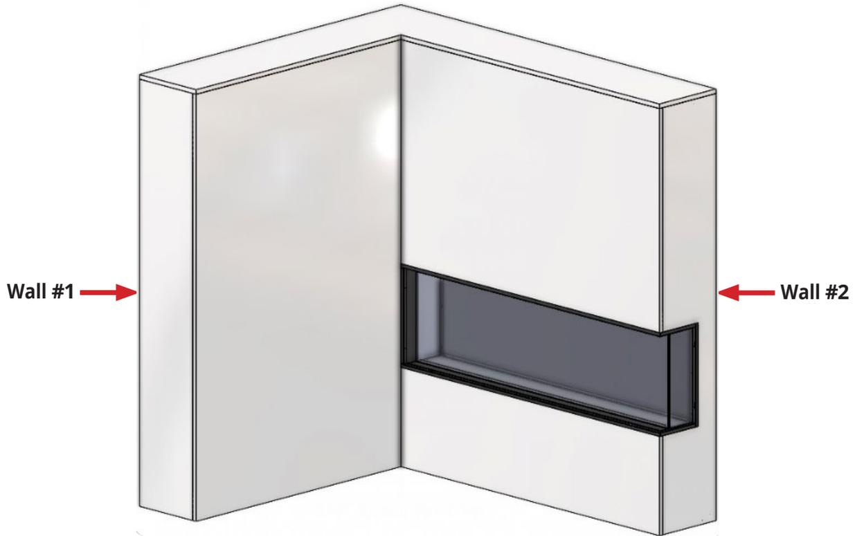
For proper fitment of the 5-piece trim, ensure that the fireplace installed in "Wall 2" has at least a 3/4" gap from the closest part to "Wall 1" as shown in the example.
