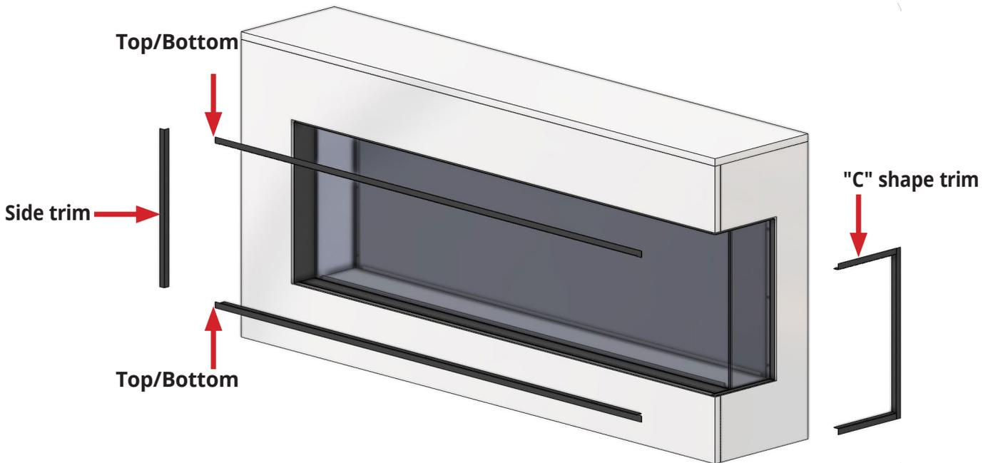
Example: Left/Right side open uses: 1 Top, 1 bottom, 1 "C" shaped, and 1 short side trim.
